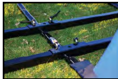
TIGHT—Spring loaded handles can be tightened by hand then quickly configured all facing down.
